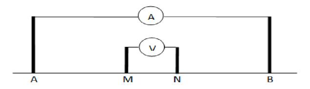
Figure 2 Schematic diagram of the schlumberger array used in the survey.
